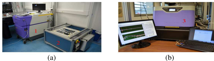
Figure 1. Photography of (a) Teraview TPS 3000 system and (b) TPS 4000 system. The TPS 4000 system is more compact and transportable.
